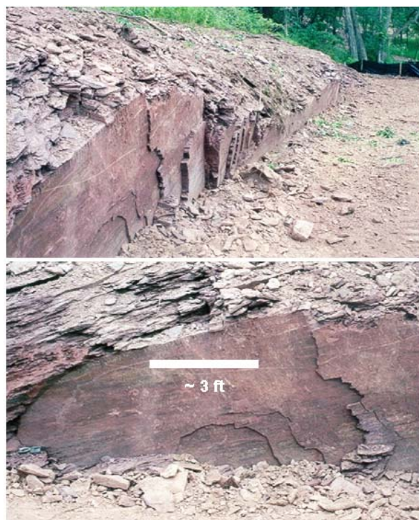
Figure F4. Joints in the Passaic Formation (location 3Q, fig. F3). Joints are elliptical, systematic extension fractures that form in clustered sets. They dip steeply and form in conjugate arrays. Photograph provided by Matthew Mulhall.
