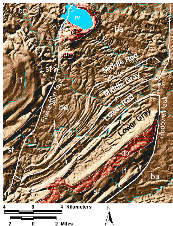
Figure F5. Shaded relief map of the Amwell Valley showing four zones in the Brunswick aquifer with contacts following pronounced topographic ridges. db – diabase, sf – Stockton Formation, lf – Lockatong Formation, ba - Brunswick aquifer, cg – conglomerate, rv – Round Valley reservoir.
