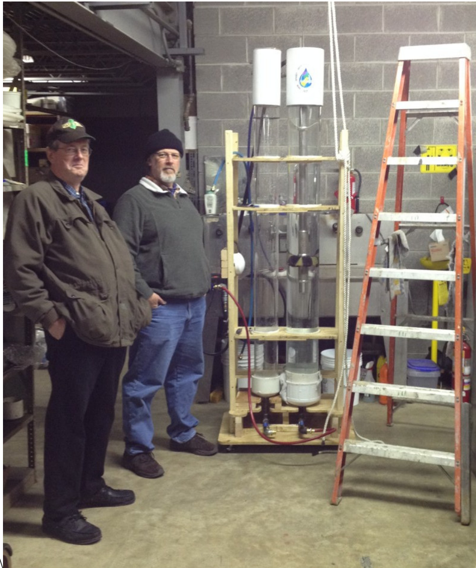
Chief James T. Boyle and coauthor Mark French oversees HFM system testing in the NJGWS garage. The HFP-2293 is positioned in the clear, 7.5-inch pipe to the right and setup for upward, low-flow testing.
