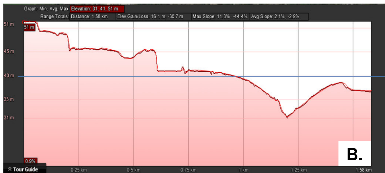
Figure 23: Google Earth (GE) was used to develop cross-section elements including a topographic profile (B.) that was auto-generated along the section trace (A.). The deviation between dip azimuth and the section trace is also highlighted in A. The GE display was captured and placed into MS PowerPoint for tracing with a freeform polyline. The profile topography requires further manipulation to place it into the project with the proper aspect because it is not captured with equal horizontal and vertical scales (1:1 scale) and therefore requires manual rescaling. This is further addressed in the Teacher's Workshop (Chapter 1).
