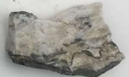
Quartz veins with mudrock seams in shear zone
