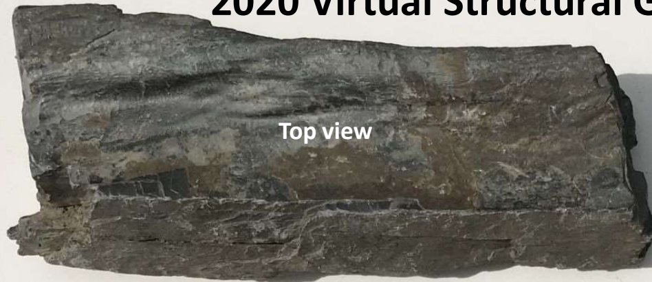
Samples of Alleghenian spaced and slaty cleavage from NJ and Eastern, Pa
