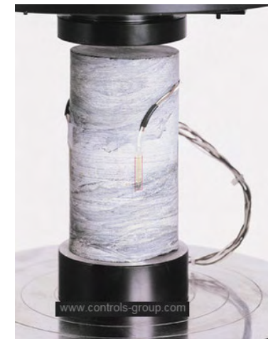
Uniaxial test with three strain gauges attached
