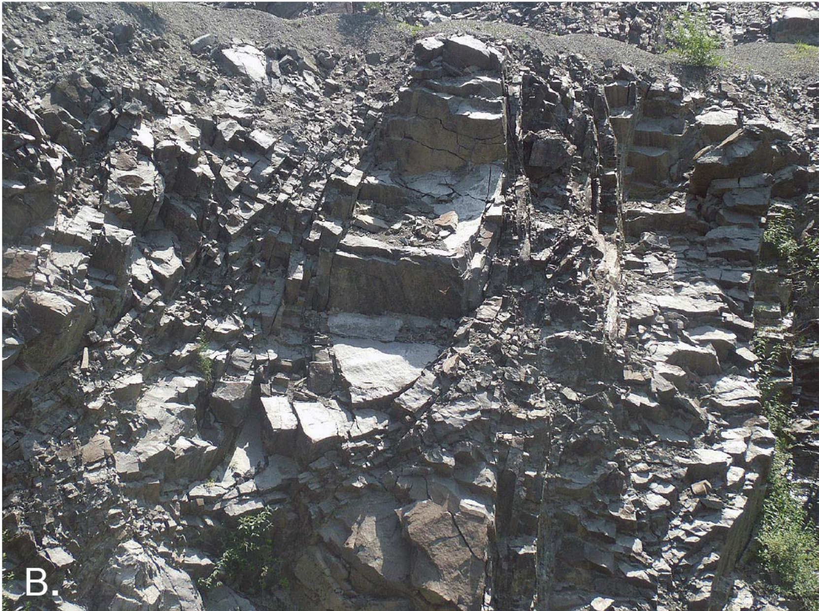
Figure 5. A. NJGS geologist measuring a small fault plane at station 67144 (slickensided shear plane - table 1). B. Anastomosing shear planes surround pods of less-fractured rock that locally impart a “watermelon seed” texture to the face cuts (station 67124)
